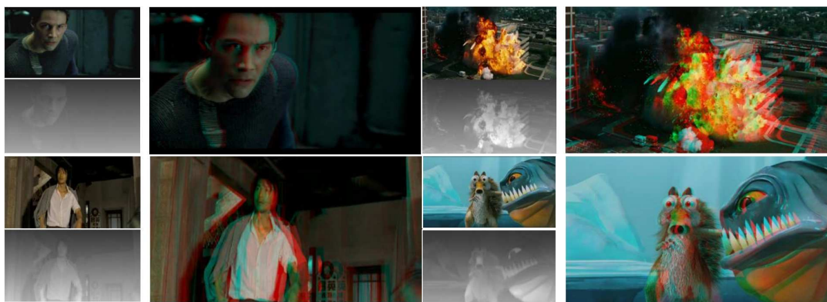
Fig. 2. Original 2D images (upper left), depth maps (bottom left), and red-cyan images (right) of test sequences.
